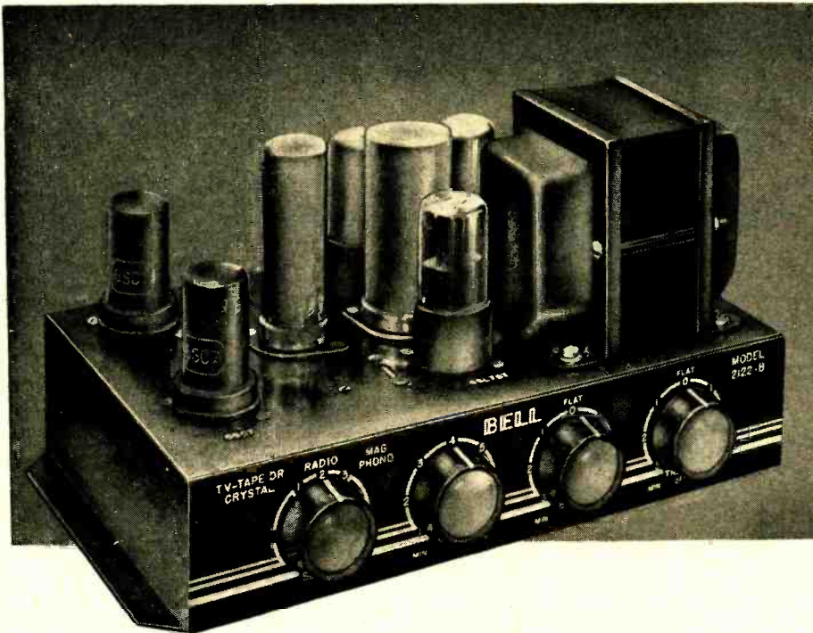
Typical high-quality audio amplifier—includes a phono pre-amp.
