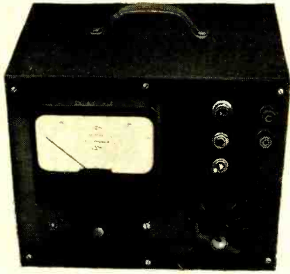
The relative field-strength meter simplifies antenna installations.
