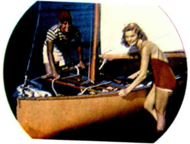
Fig. 13—Failure of "Q" signal produces reddish picture.
