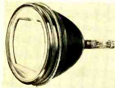
Three-gun tricolor picture tube 15GP22.
